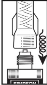
Attach proper mixing nozzle supplied by the manufacturer to the cartridge. Do not modify nozzle.
