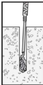
Fill hole approximately 2/3 full, starting from bottom or back of the cleaned drilled hole. Withdraw the nozzle slowly to avoid creating air pockets.
