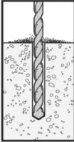
Drill hole to specified diameter and embedment depth.
