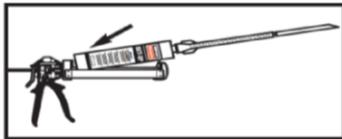
Insert cartridge into the appropriate dispensing tool.
