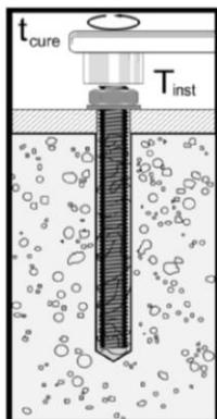
After required curing time  $t_{\text{cure}}$  anchor can be loaded. Apply the installation torque  $T_{\text{inst}}$  using calibrated torque-wrench.
