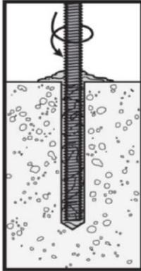
Insert clean, oil free anchor, turning slowly until the anchor contacts the bottom of the hole.
