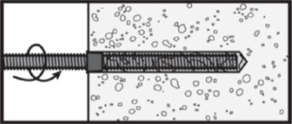
Insert clean, oil free anchor, turning slowly until the anchor contacts the bottom of the hole.
