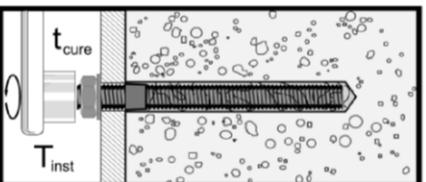
After required curing time  $t_{cure}$  anchor can be loaded. Apply the installation torque  $T_{inst}$  using calibrated torque-wrench.
