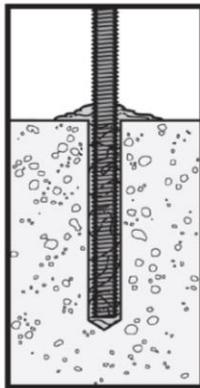
Do not disturb the anchor until fully cured. The curing time  $t_{\text{cure}}$  is given in table B3.
