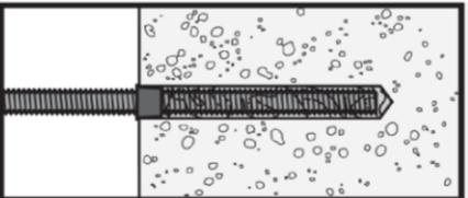
Do not disturb the anchor until fully cured. The curing time  $t_{cure}$  is given in table B3.
