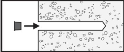
Install adhesive retaining cap.
