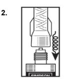
Attach proper mixing nozzle supplied by the manufacturer to the cartridge. Do not modify nozzle.
